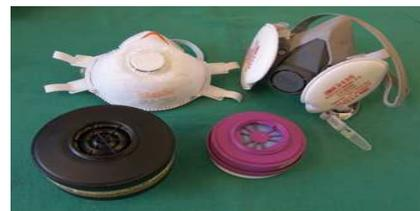
For electrostatic respiratory filters, the most penetrating particle size (MPPS) is around 30 nm: standardized measurement tests should be adapted from 600 nm to 30 nm. In **dry condition**, the penetration of nanoparticles decreases with time. With **humidity brought by breathing**, the penetration of nanoparticles through the electrostatic media increases, close to the threshold value (1%) defined for the FFP3 mask (NF EN149) after 2 hours of usage.
