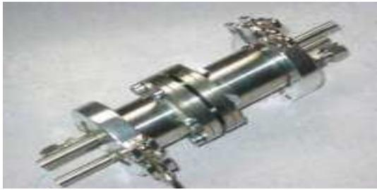
The "through diffusion method" derives from standard NF EN ISO 6529 and NF EN 374 uses a diffusion cell in which a constant particle concentration is imposed in the upper flow part. Diffusion coefficients are calculated from the measurement of nanoparticle flowing in the down flow part of the cell.
