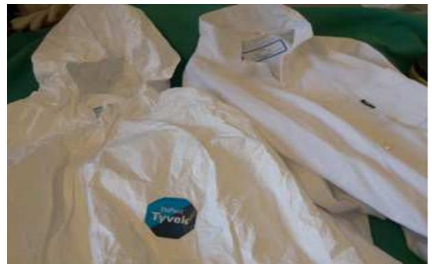
Tests performed with graphite nanoparticles centred at 40 nm and 80 nm showed that high density polyethylene textile (Tyvek® type) seems to be better than cotton and polypropylene.
