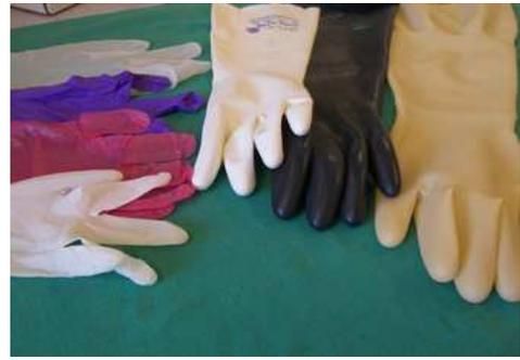
Several types of gloves have been tested by Helium diffusion test. All the tested gloves are made of porous material which differs according to the material and thickness. On the other hand, after exposure to a high concentration of graphite aerosols, ranging from 20 to 100nm, no particle penetration can be measured.
