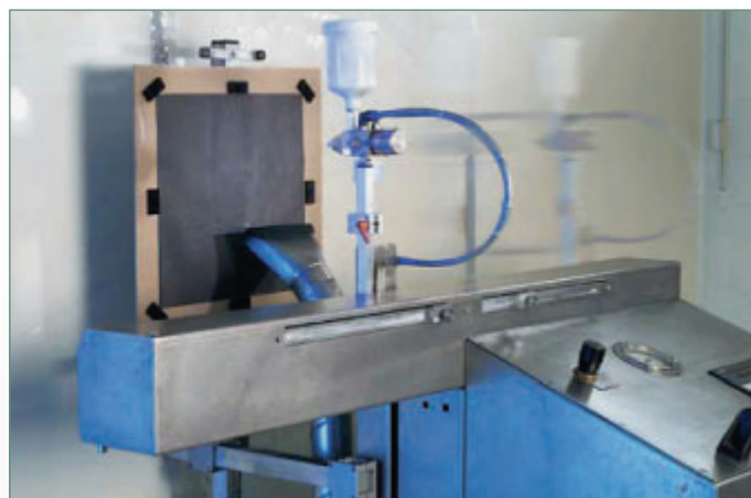
Figure 1 Ink-jet equipment pulverizing nanoparticles for battery electrodes (Source: CEA).
