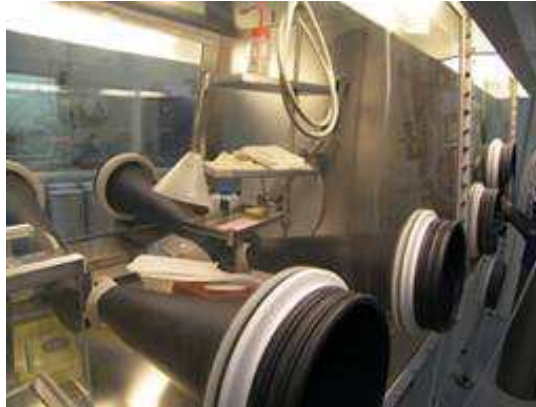
Glove box & HEPA filter on Nanomil workshop CEA DRT
